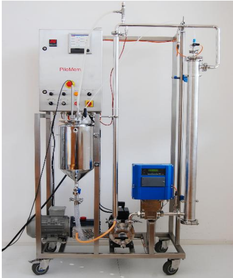
Lab scale Nano filtration pilot plant (2,6 m 2 )
